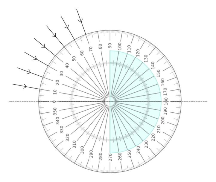
Place a semi-circular block over the blue area. Make sure the centre of the flat face is over the cross in the middle of the circle. Direct rays of light along each of the black arrows, and record your observations in the table below.
